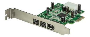
This 3 Port PCI Express FireWire adapter card can be installed in a PCI Express slot to add two IEEE1394b (FireWire 800 - 9 pin) ports and one IEEE1394a (FireWire 400 - 6 pin) port, providing broad compatibility with a wide range of FireWire devices (e.g. DV camcorders, external hard drives, digital cameras, etc.).
